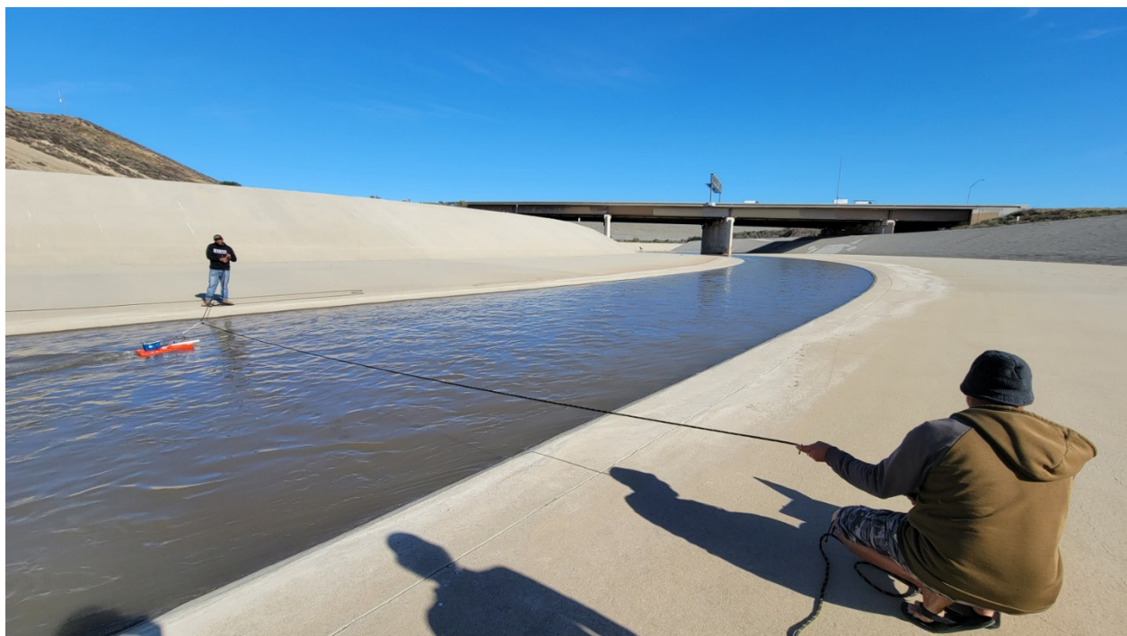
Figure C-18. USGS staff performing ADCP field measurements at SAP.
