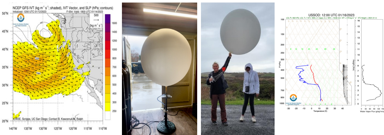
Figure C-9. (left) Integrated Vapor Transport (IVT) forecast for the one of the ARs that impacted the US West Coast in mid-January. (middle left) A helium-filled meteorological balloon prior to launch at USSOD. (middle right) L. Katz and family friend ready to release a radiosonde from USBOD. (right) Highest IVT for this storm recorded at USSOD. These figures are created for each launch and can be found in the Drive folder, linked below, under the launch location and within the Skew-T folder.
