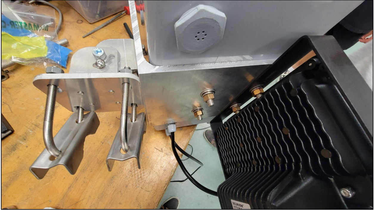
Figure C-22. Security enclosure mount, mast bracket, and IR illuminator mount
