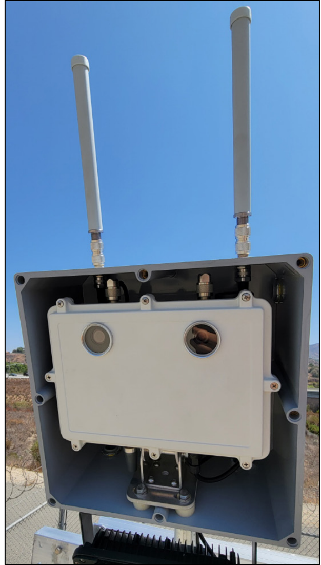
Figure C-24. (left) CW3E fabricated antenna connectors connected to CVSG (right) Antenna connectors connected to antenna feed-throughs and antennas.
