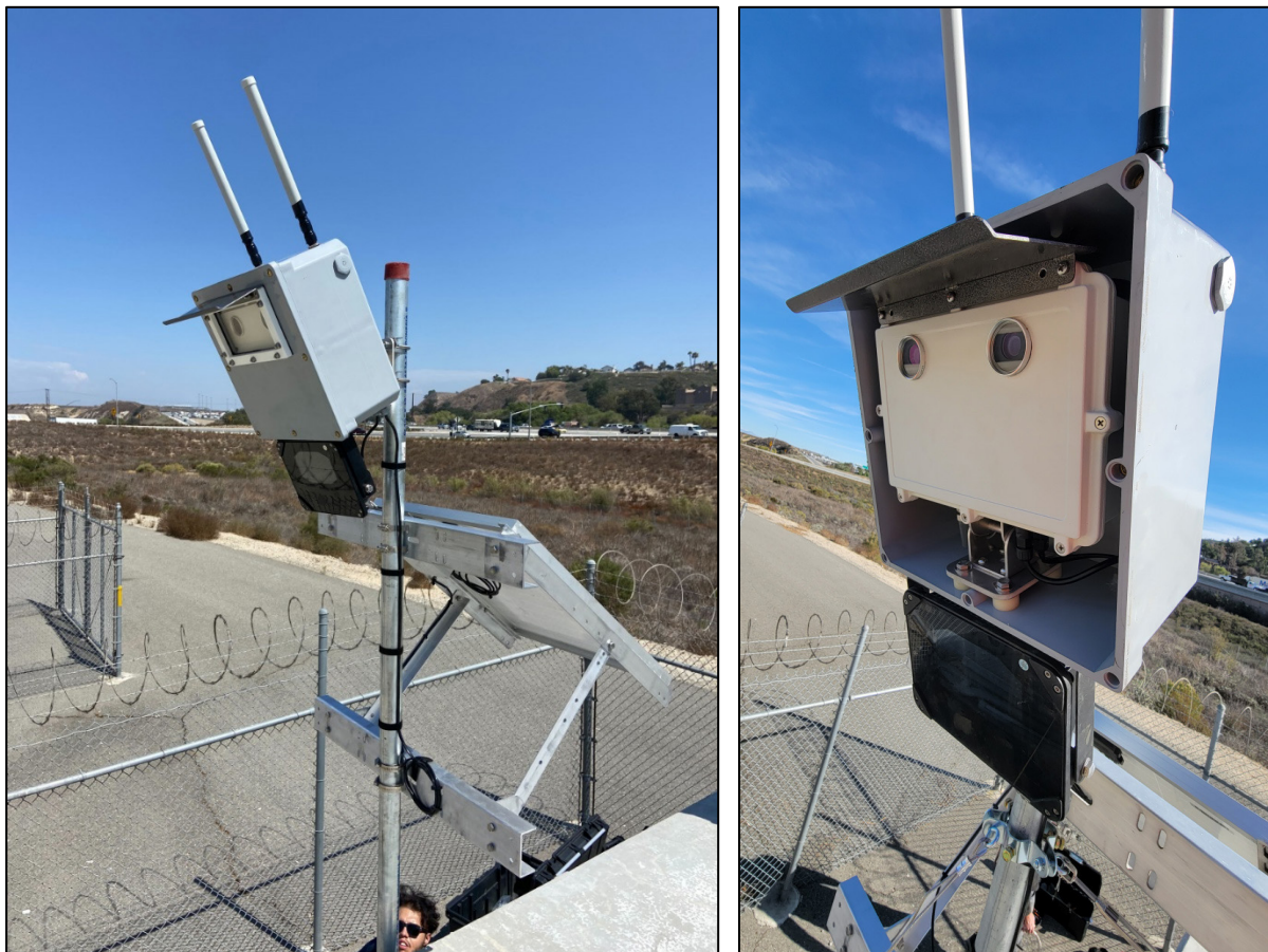
Figure C-30. (left)). Security enclosure faceplate installed on CVSG. (right) Security enclosure faceplate removed November 17th, 2022 to minimize droplet distortion.
