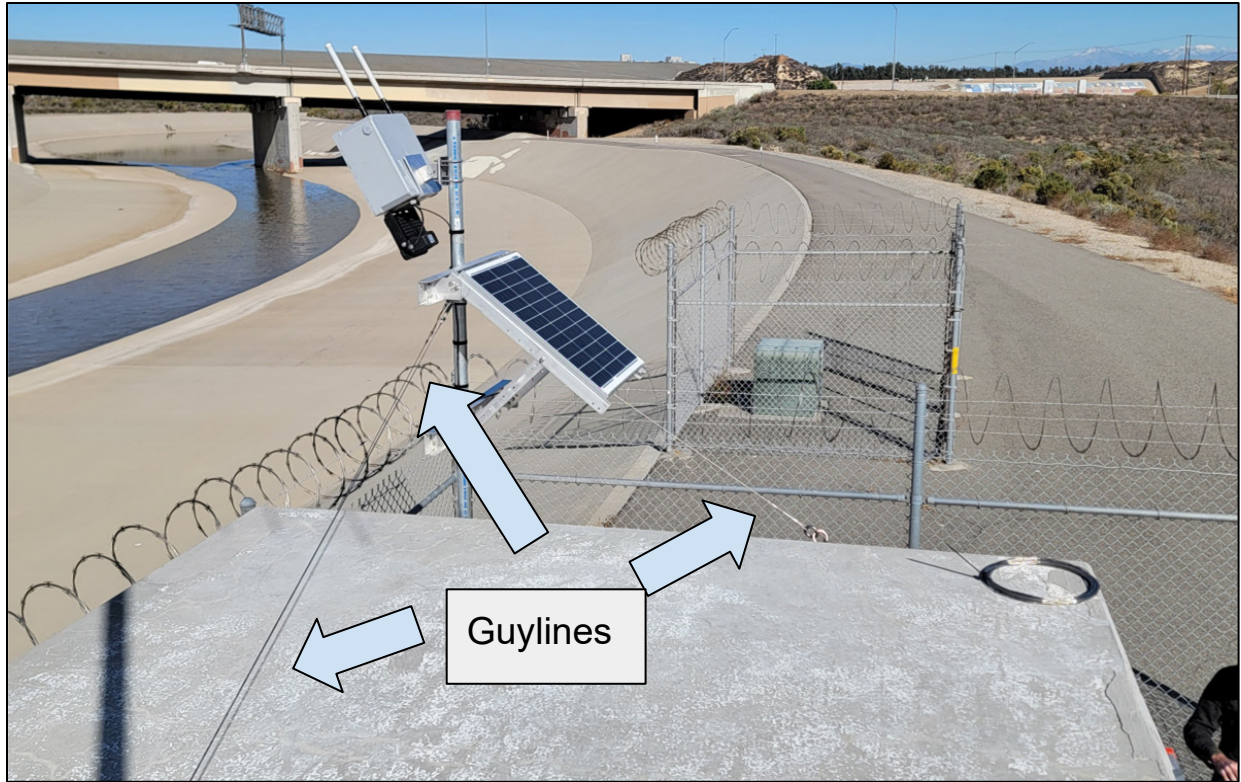
Figure C-32. Guylines were installed in November 2022 to minimize mast movement in high winds.
