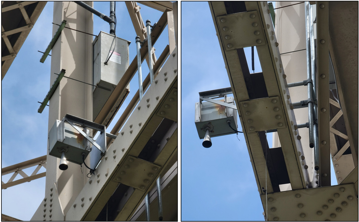
Figure C-49. USGS Design Analysis H-3611 radar sensor installed at MWD Pipeline crossing.
