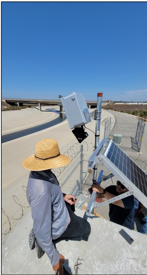
Figure C-29. CVSG, security enclosure, IR illuminator, and solar panel were attached to the 1.5" mast using U-bolts.
